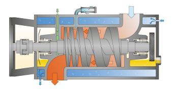
The machine works on the one-stage, twin-screw pump principle.
