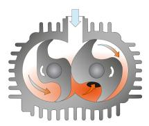
The machine works on the claw principle.
