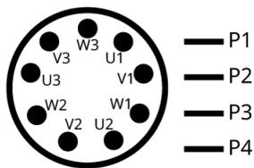
Connection of motor temperature switches (recommended):
