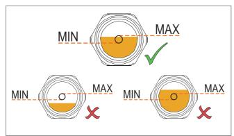
If the oil level does not reach the target circle level:
